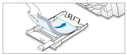
5. Slide both paper adjusters in until they stop at the edges of the paper. Make sure that the paper stack lies flat in the tray and that the paper fits under the tab of the paper-length adjuster.
